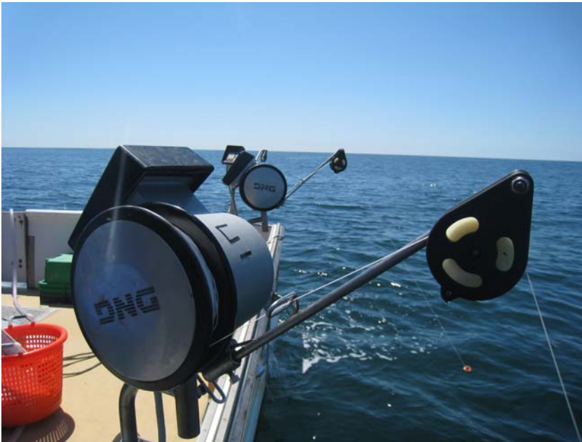
Figure 5. Jigging machines installed on F/V Andanamara. Three machines were deployed off the port rail and stern quarter.
