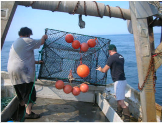
Figure 7. Norwegian two-chamber pot being deployed on the F/V Bad Penny.
