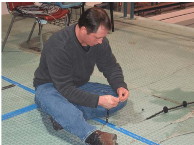
Figure 5. Capt. Vincent Balzano, the industry partner working on a model trawl wire at the shooting deck of the flume tank.
